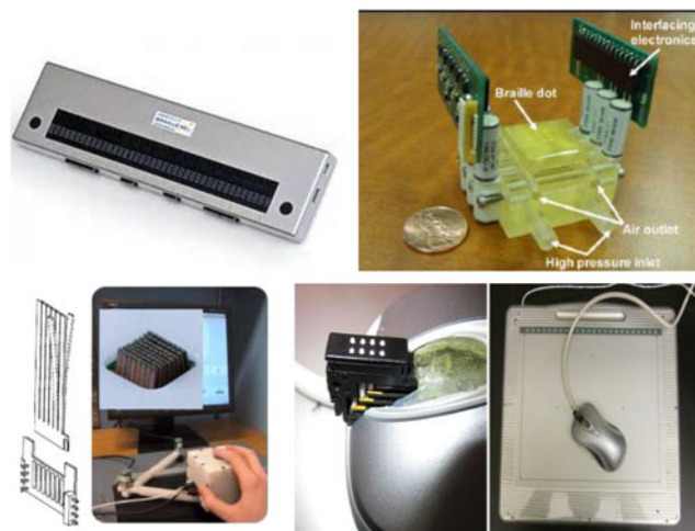
Fig. 5. Top left, typical commercial Braille display (from [96]); Top right, microbubble actuator (from [92]); Bottom left, laterotactile display with pentagraph device (used in Levesque et al. [94]); Bottom right, Braille cell with graphics tablet (used in Headley et al. [97]).
