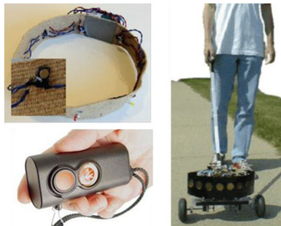
Fig. 7. Top left: Vibrotactile belt that has been used for either navigation or obstacle avoidance, from [128]. Bottom left: using the Miniguide. Right: Guidecane, from [142].
